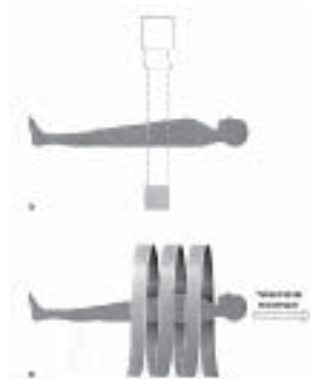
Fig-2, Depicts volumetric acquisition of data in a spiral scan (Image courtesy intl.elsevierhealth.com/ebooks/pdf/aw.pdf)
